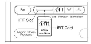
Next, select the desired program on the iFIT Card by pressing the up and down buttons next to the iFIT slot.
